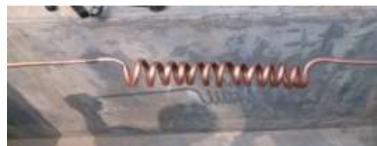
Fig 2: fabrication of helical coil heat exchanger
