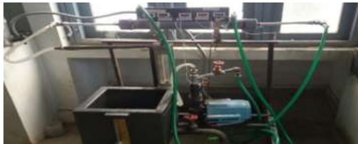
Fig 3: Experimental setup of helical coil heat exchanger with supporting instrumentation.
